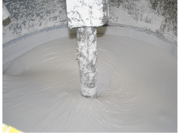
Figure 2 shows a picture of a choked vortex
